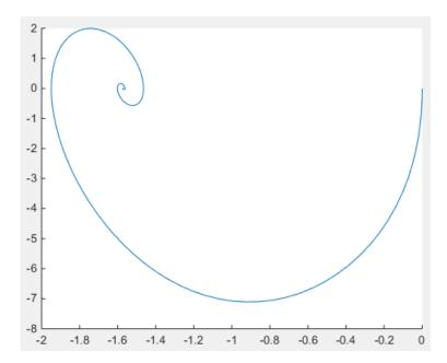
Try simulating the model using different starting angles. You can change the starting angle in the **State Targets** > **Position** menu of the Revolute Joint block dialog box. The figure shows a compound phase plot for starting angles of -240, -180, -120, -60, 0, and 60 degrees.
